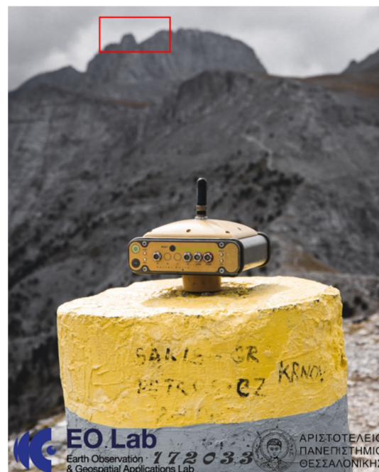
Fig. 4 GNSS receiver at NTN benchmark and the Mytikas peak in background (red frame).
